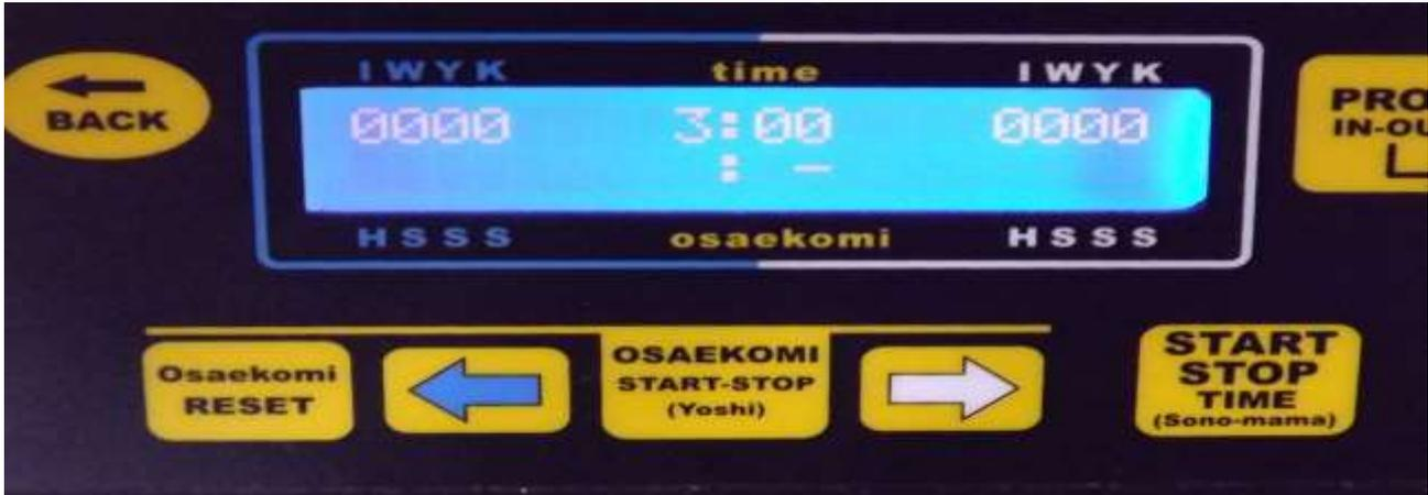
Press the "**START STOP TIME**" key and this will start the backward count of the contest time. The start of this operation does not start the Osaekomi time. The time is stopped by again pressing the "START STOP TIME" key. When the time count is stopped, the 2 separation points minutes/seconds light up continuously, otherwise they keep on flashing.
