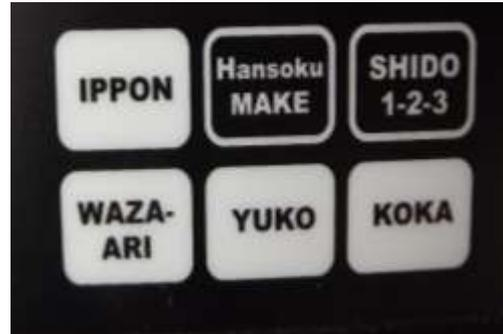
With the, "**KOKA**", "**YUKO**", "**WAZA-ARI**" and "**IPPON**" keys, the scores are incremented accordingly. In the case of "**KOKA**", and "**YUKO**", after 9 the following letters appear A (= 10), B (= 11), C (= 12), D (= 13), E (= 14), F (= 15).
